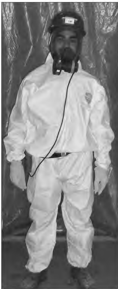
Powered air-purifying respirator
