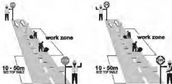
Typical Arrangement on Two-lane Roadway
