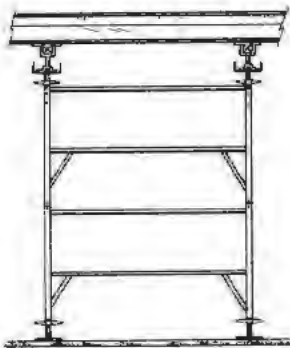
Figure 207 Typical Shoring Tower with Stringers, Adjustable Base Plates, and U-Heads
