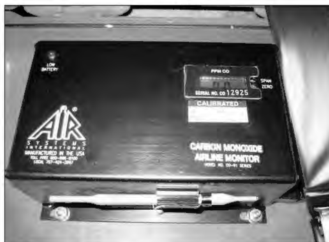
Carbon monoxide monitor
