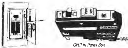
GFCI in Panel Box
