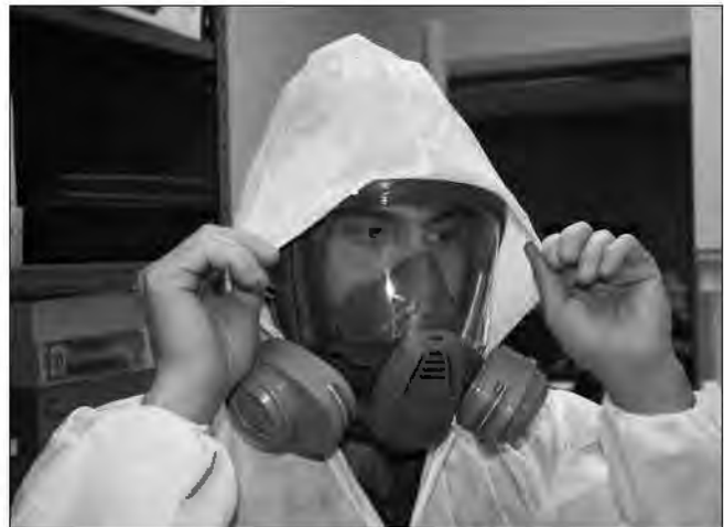
Full-facepiece non-powered air-purifying respirator
