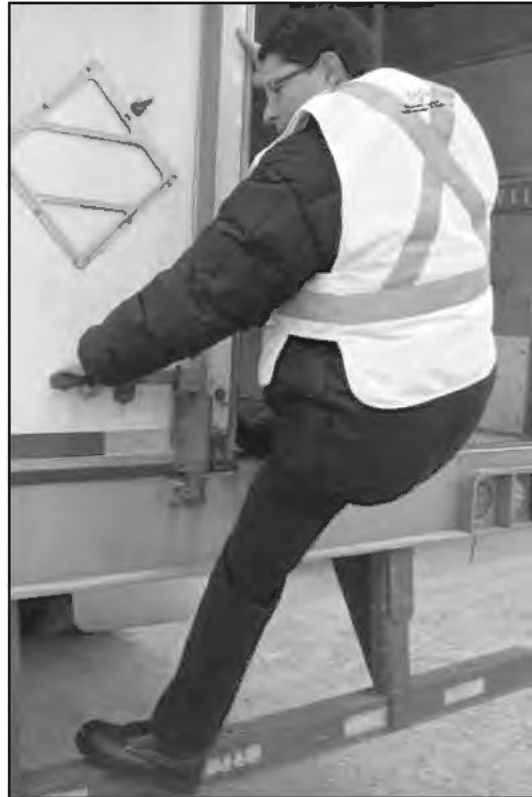
Figure 6: Always use three-point contact when mounting and dismounting from vehicle.
