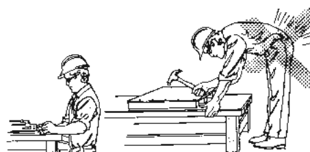
For bench work, the right height is vital.
