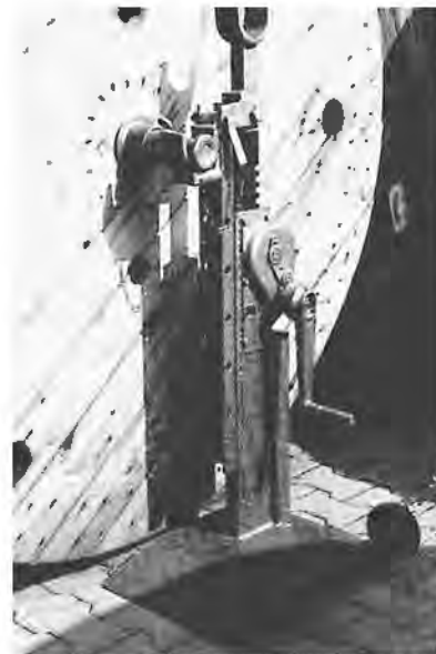
The rack bar should always be greased, except on the toothed side
